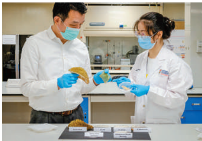
Prof William Chen and PhD student Cui Xu holding their hydrogel bandage made from durian husk. (Photo credit: Professor William Chen)
